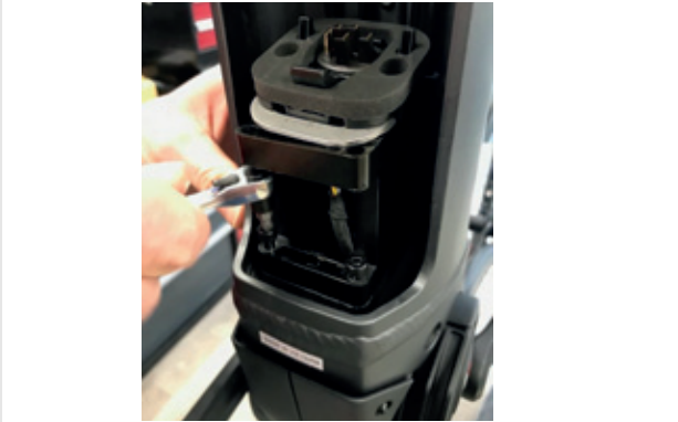
Figure 23: Removing the 4 mm hexagon screws
