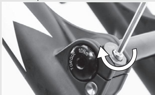
Figure 33: Tightening the securing clip
