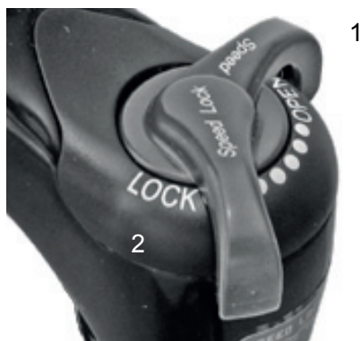
Figure 64: Suntour compression adjuster with OPEN (1) and LOCK (2) positions
