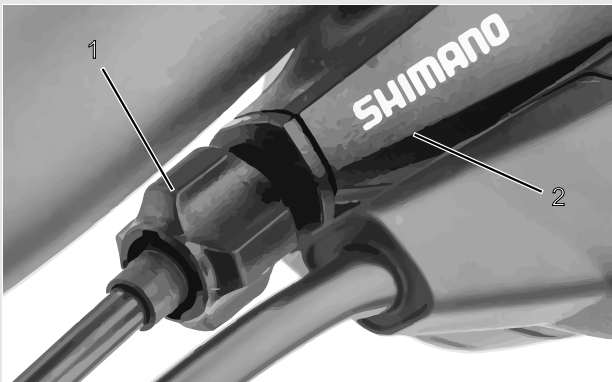
Figure 69: Adjusting sleeve (1) for the single-cable, cable-operated gear shift with shifter housing (2), example
