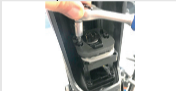
Figure 22: Undoing screws on battery mount
