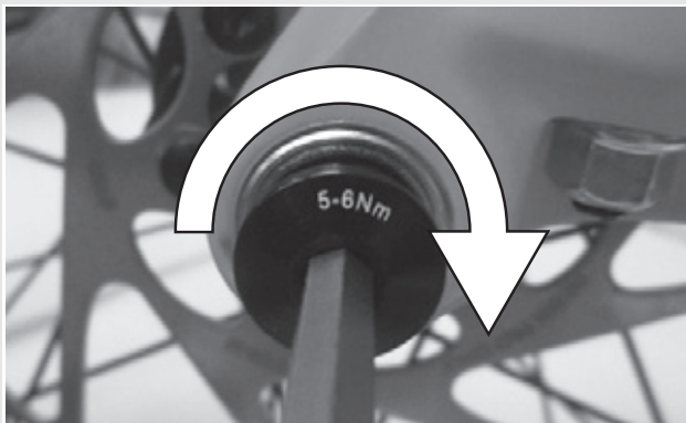
Figure 31: Tightening the securing screw
