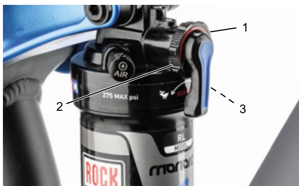
Figure 79: Setting the rebound damper strength on the rear frame damper setting wheel (1)
