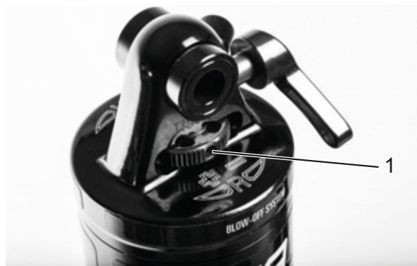
Figure 61: Suntour rebound adjuster wheel (1) on the rear frame damper
